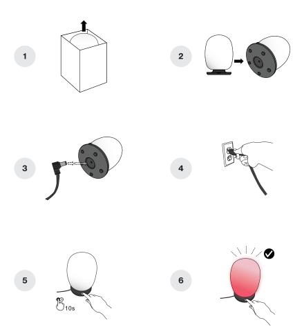
Insert AC plug of power supply unit into a wall outlet with a voltage between 100V and 240V. (Standard US residential voltage is 120V).
